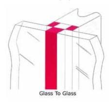
Recommended for use in many forms of construction including glass to glass joints, curtain wall assemblies, perimeter seals on curtain walling, perimeter sealing of polyester powder coated and PVCu frames and glazing of windows in swimming pool buildings.
